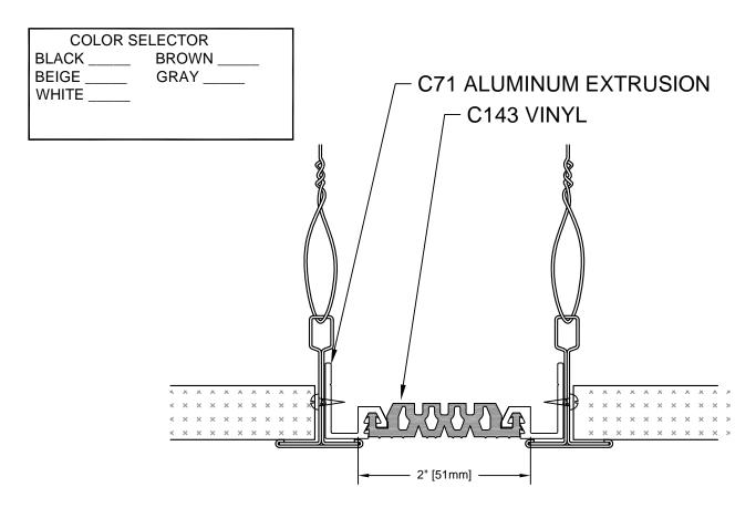
DESCRIPTION: CEILING TO CEILING ALUMINUM: 6063-T5 EXTRUSION
