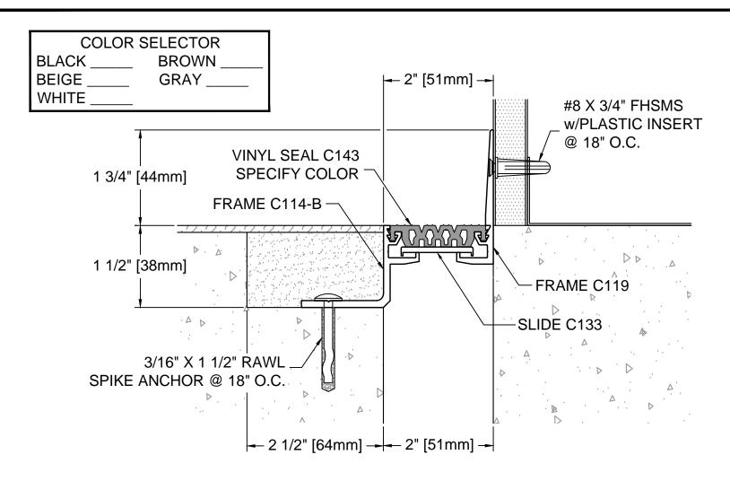
DESCRIPTION: FLOOR-TO-WALL ALUMINUM: 6063-T5 EXTRUSION
