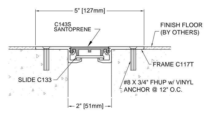
DESCRIPTION: FLOOR-TO-FLOOR ALUMINUM: 6063-T5 EXTRUSION
