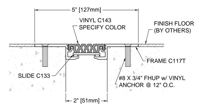
DESCRIPTION: FLOOR-TO-FLOOR ALUMINUM: 6063-T5 EXTRUSION
