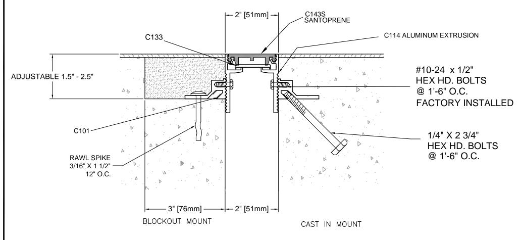
**DESCRIPTION: FLOOR-TO-FLOOR** ALUMINUM: 6063-T5 EXTRUSION
