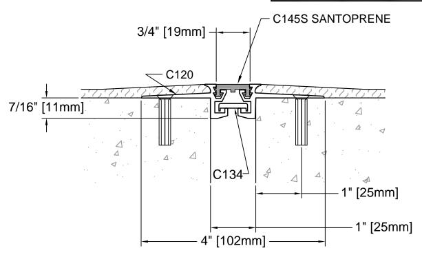
**DESCRIPTION: FLOOR-TO-FLOOR ALUMINUM: 6063-T5 EXTRUSION**
