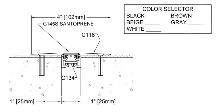
DESCRIPTION: FLOOR-TO-WALL ALUMINUM: 6063-T5 EXTRUSION
