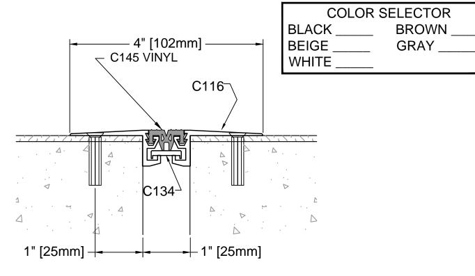
DESCRIPTION: FLOOR-TO-WALL ALUMINUM: 6063-T5 EXTRUSION
